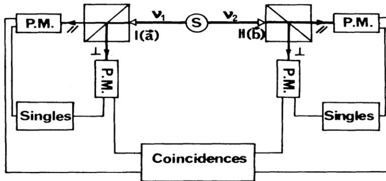
Note: Two polarizers I and II, in orientations a and b, performed true dichotomic measurement of linear polarization on photons  $v_1$  and  $v_2$ . Each polarizer is rotatable around the axis of incident beam. The counting electronics monitors the singles and the coincidences. This graph is taken from the article.
